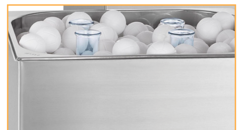
Ball Shield - Polypropylene spheres act as a barrier between the liquid and the air.
