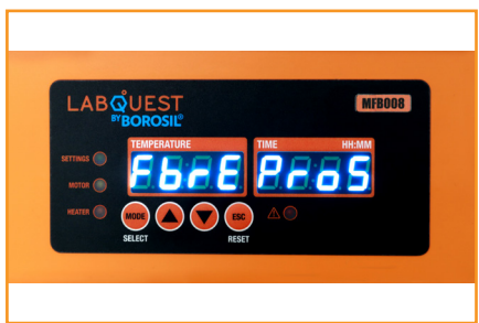
Buzzer alert upon process completion
