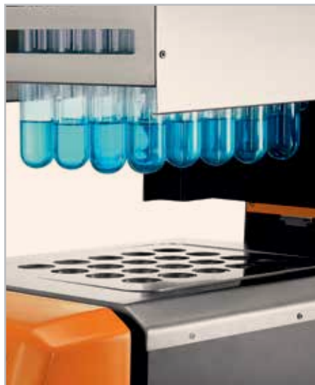
The tube rack with manifold is automatically lowered into the digester and can be lifted automatically in between to check the completion of digestion
