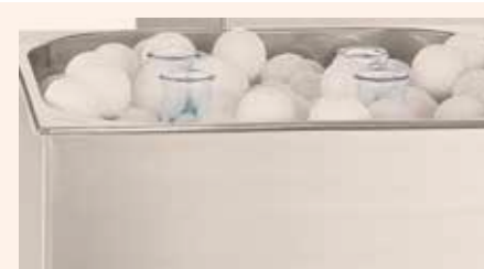
Ball Shield anti evaporating spheres
