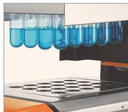
The tube rack with manifold is automatically lowered into the digester and can be lifted automatically in between to check the completion of digestion
